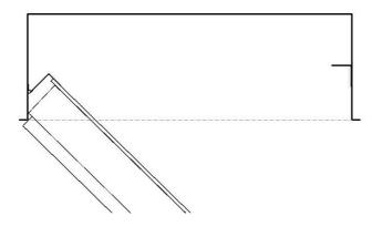
The other problem is that as the panel swings forward the assembly hits the side of the box limiting the opening angle.
