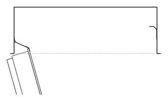
As can be seen here the double hinge now allows the panel to open and give easy access to the rear of the panel.
