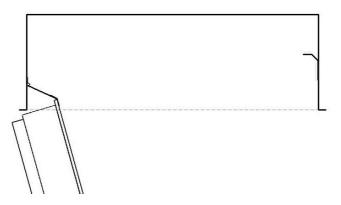
As can be seen here the double hinge now allows the panel to open and give easy access to the rear of the panel.
